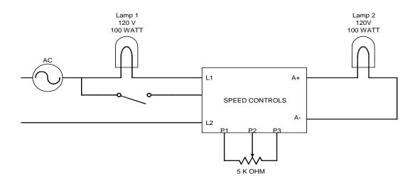
Be sure SPST switch is in OPEN position and 5K pot is set fully CCW. Be sure to replace plug-in-resistor. Apply line voltage. If control is good, lamps 1 and 2 should be dim or off. If lamp 1 is at full brightness, then there is a short circuit in the Power Bridge of the KBIC control. Remove control from test and repeat Step 2 (A)-(E).
