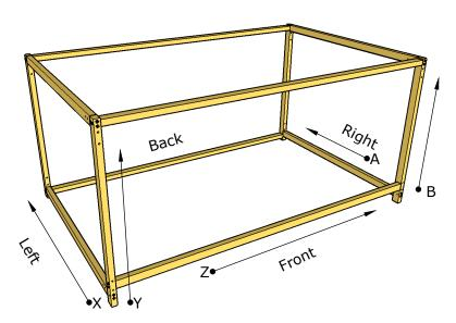
Having four independent axes allows to cut also non square objects like tapered model airplane wings.
