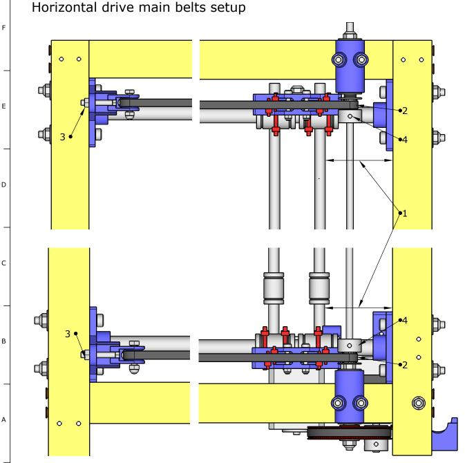
Make sure the 18 teeth pulleys are free to move before starting.
