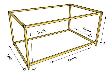
Having four independent axes allows to cut also non square objects like tapered model airplane wings.
