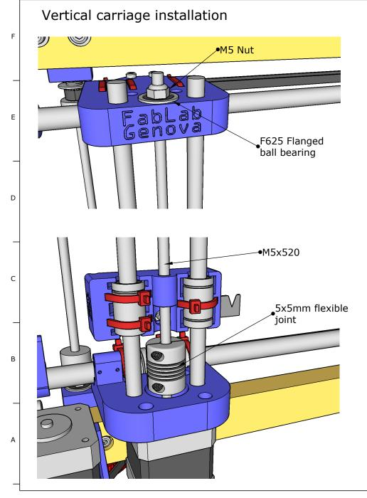
Slide the 5\*520 threaded rod through the upper carriage, screw through the cursor and fix it to the flexible joint. Insert the flanged bearing on the upper carriage and screw in the retaining nut - it has to be tighten so it just touches the bearing.
