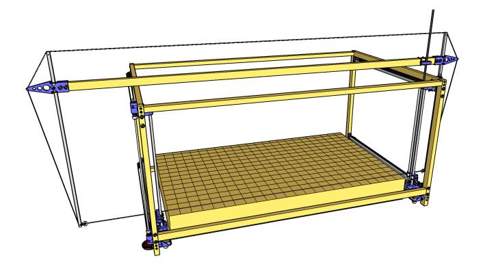
4 axis, cheap, modular CNC hot wire foam cutter
